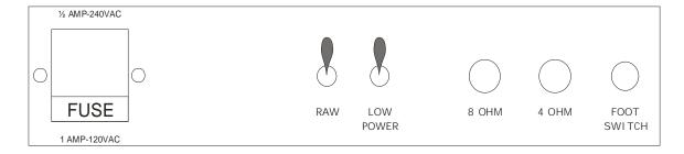
There are 2 voicing switches on the back panel. Along with the speaker jacks and the jack for the Reverb foot switch.
