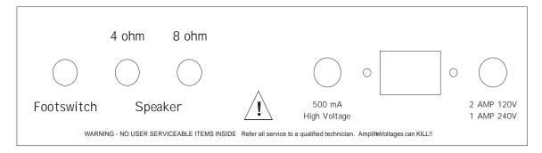
The speaker jacks and the jack for the Tremolo foot switch are on the back panel.
